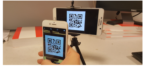
Fig. 4. Usecase: a user captures an image shown on the verifier's interface to be authenticated (or registered).
